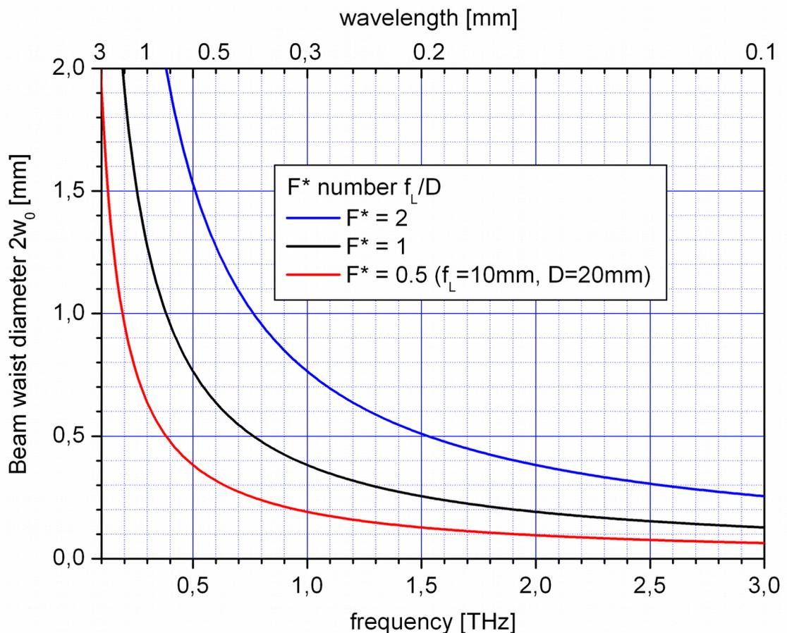
Figure 1: Calculated focus diameter  $2w_0$  as a function of THz frequency according to equation (1)
