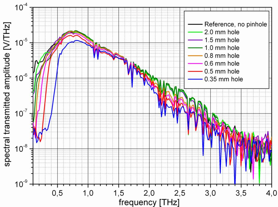
Fig. 4: Measured spectral transmission through pinholes with different hole diameters.  $F^* = 0.5$
