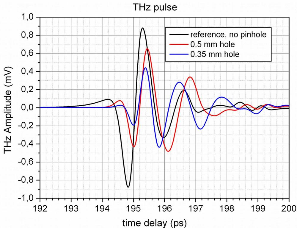
Fig. 3: Measured pulse amplitude after pinholes with diameter 0.5 mm and 0.35 mm
