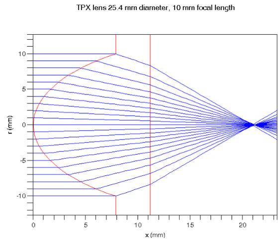
Focusing TPX lenses: Focal length  $f_L = 10$  mm
